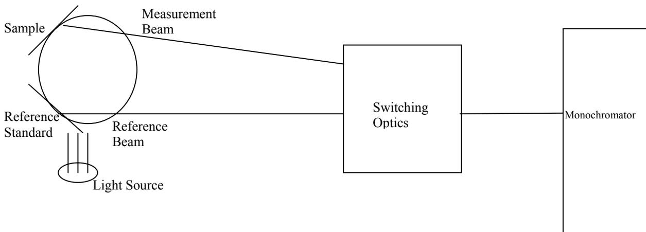
In the double beam configuration, fluctuations in the light source, detector, or electronics, and changes in the sphere are removed from the measurement each time a measurement is taken.
