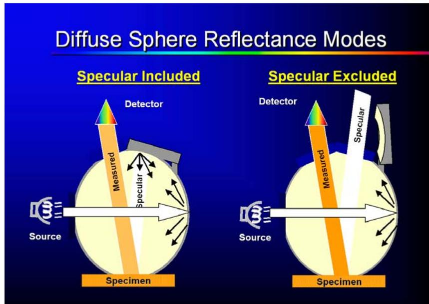
These images show what the two modes look like inside the transmission compartment of a ColorQuest XE, UltraScan XE, UltraScan VIS or UltraScan PRO.
