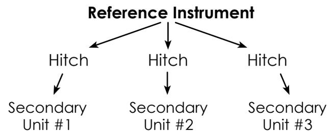
Here's a simple example: Reference instrument was used to read a standard. It was then hitched to another instrument and the standard was read again. The values read on the reference instrument are shown in Table 1 and the results as expected indicate that the readings after hitch standardization are closer to the reference instrument readings than before hitch standardization.
