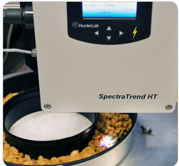
Figure 1. SpectraTrend measuring the color of honey roasted peanuts.
