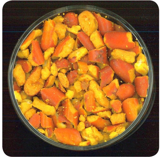
Figure 2. This is the instrument view through the bottom of the dish. The instrument optically averages all colors within the field of sample view.
