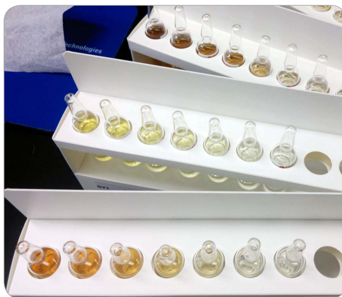
Figure 1. The 10 ml full set of EP liquid color standards from Fluka Analytical of Sigma Aldrich www.sigmaaldrich.com
